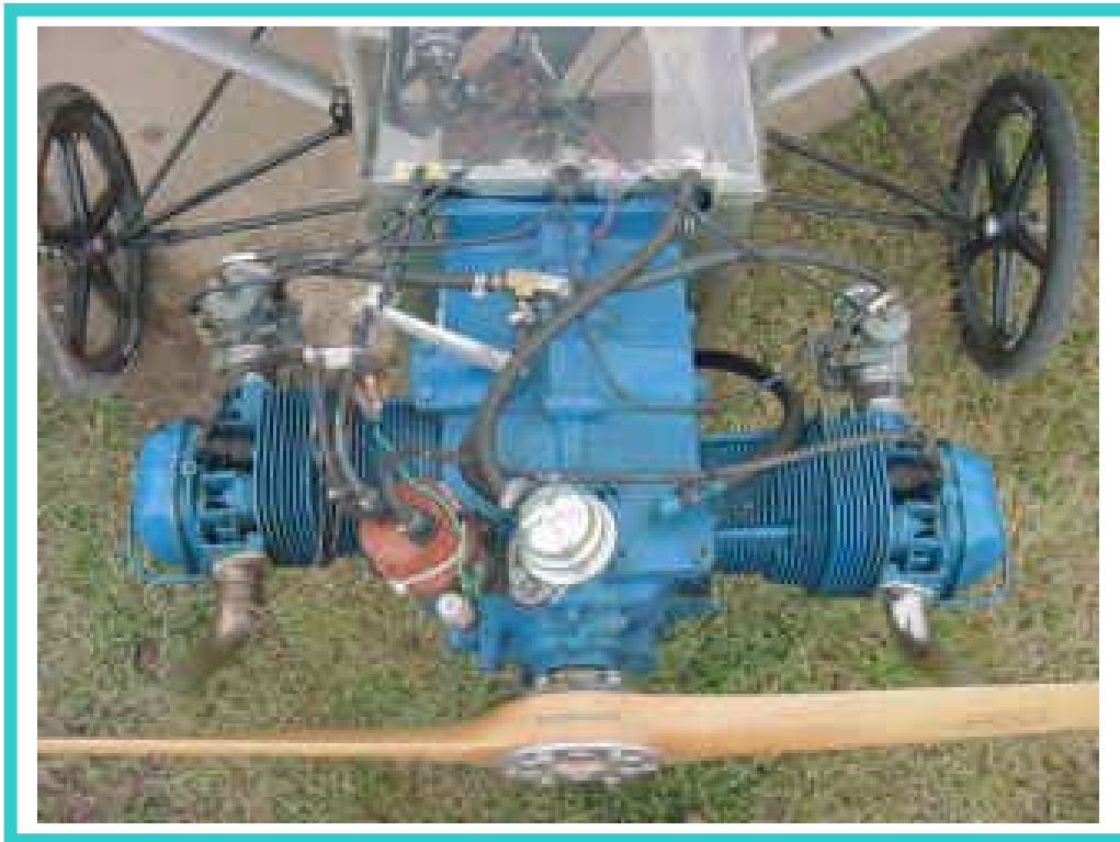
Picture: full uncut VW engine case, 1/2VW motor
